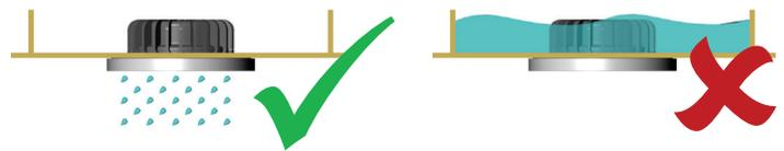
Also, it is important that the lights are mounted with airspace around the heat sink housing to allow for convective cooling of the lights. We recommend a distance of 1/2" (13mm) of free space above the housing.
