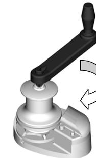
Fully tighten retrieve the anchor under power
