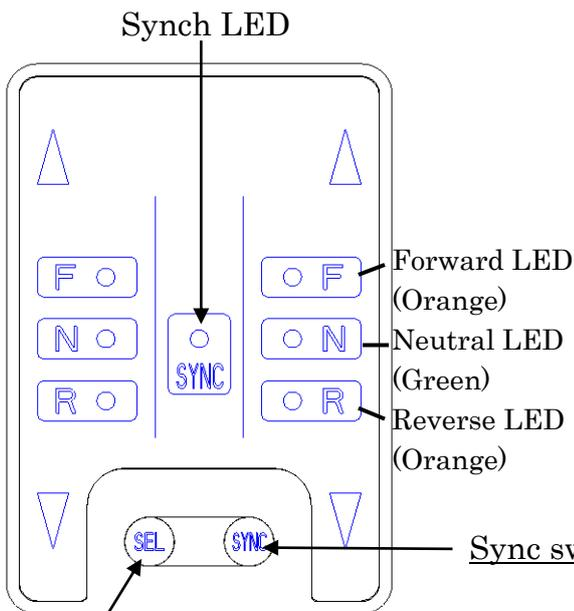
Neutral (N) LED flashes during neutral throttle operation. LED's flash when an alarm is activated.
