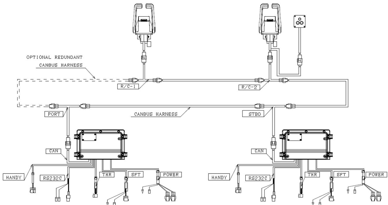
Note: The figure above is an example of a two engines / two control stations system.
