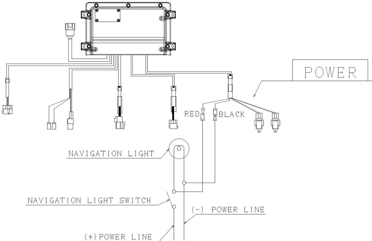
Note: Once dim harness is connected; brightness of the control head LED's illumination will be reduced whenever navigation light is ON.
