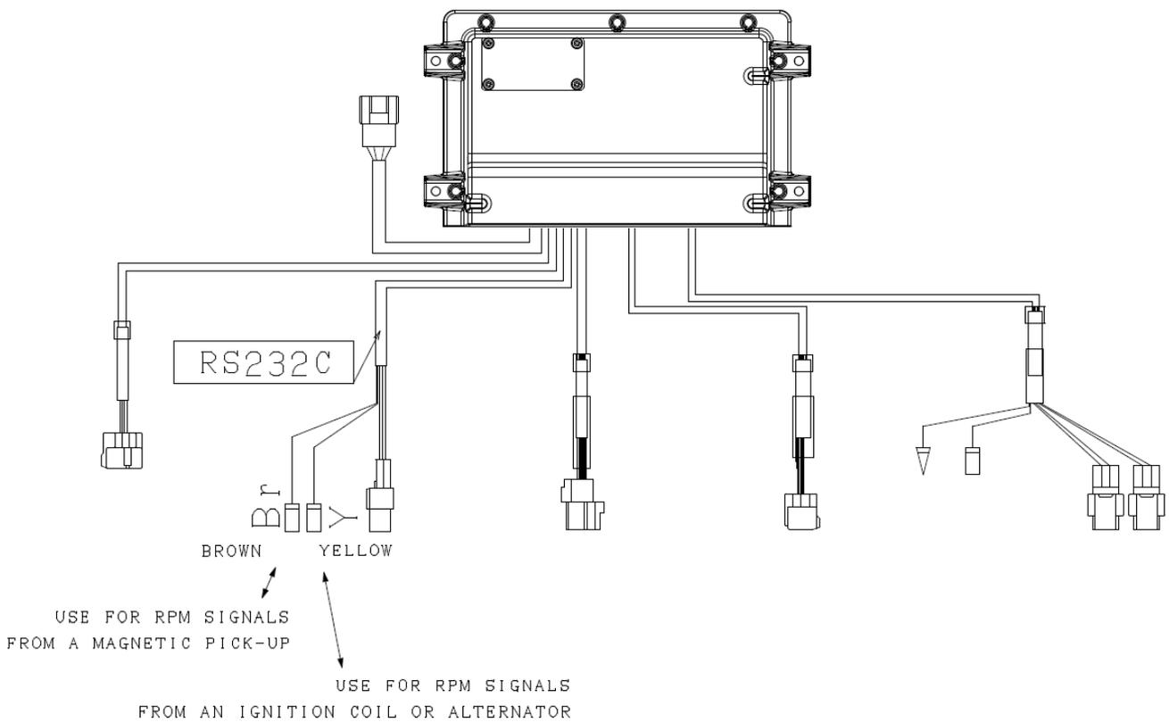
Note: No damage will occur if the case of a wrong connection; synchronization will simply be ineffective.
