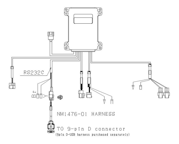
$\underline{\text{Note}}$ : Above drawing shows NM1476-01 harness & D-USB extension harness connection to KE-4XG control unit
