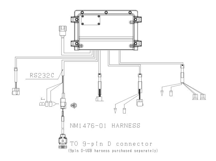
$\underline{\text{Note}}$ : Above drawing shows NM1476-01 harness & D-USB extension harness connection to KE-5XG control unit
