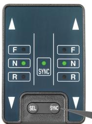
A built-in synchronization function switch (on lever) for multi-engine configurations (dual, triple, quad) eliminates the need for a separate synch kit, thus reducing installation space & wiring requirements.
