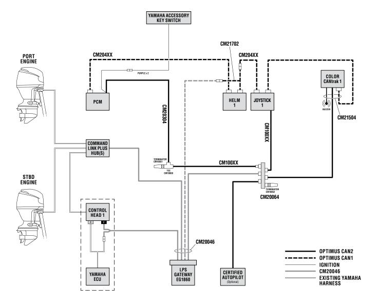
Figure 6-17. Yamaha EX – single station, twin engine.
