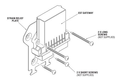
Figure 7-5. Gateway with strain relief plate.
