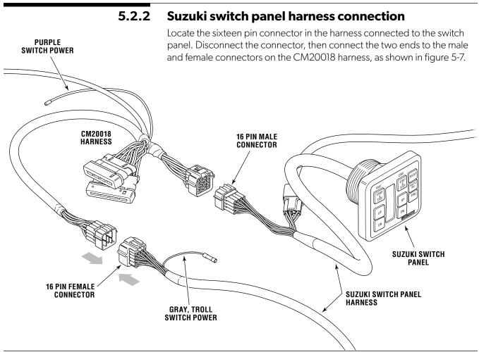
Figure 5-7. Switch panel harness connection.
