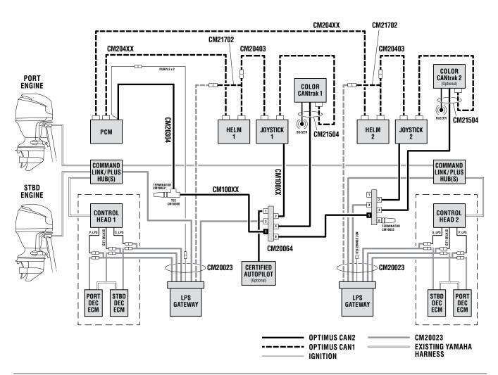
Figure 6-9. Yamaha EST – CAN2 interconnection, dual station, twin engine (with preferred CAN1 cabling).
