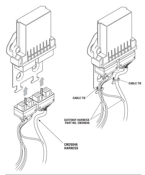
Figure 6-16. Harness connection to EST gateway.
