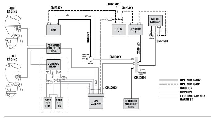
Figure 6-8. Yamaha EST – CAN2 interconnection, single station, twin engine.
