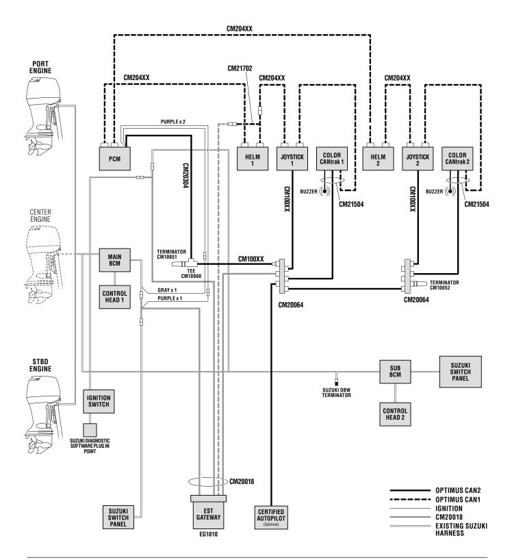
Figure 5-3. Suzuki EST dual station, twin or triple engines.
