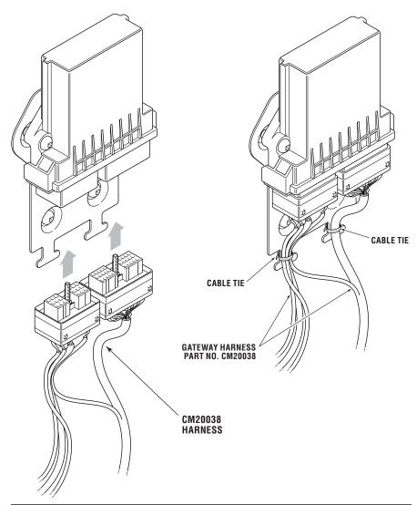
Figure 7-6. Harness connection to EST gateway.
