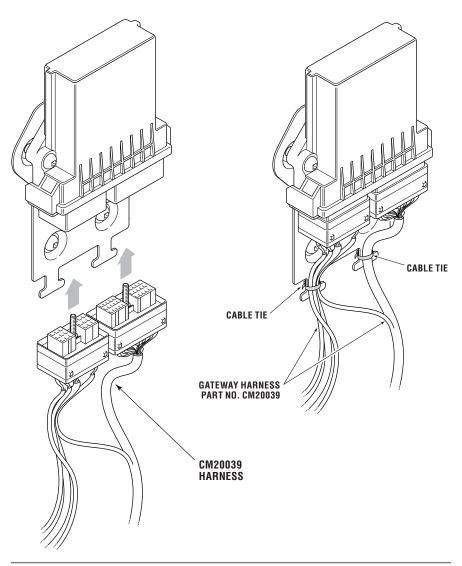
Figure 8-5. Harness connection to EST gateway.
