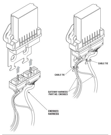
Figure 6-7. Harness connection to EST gateway.
