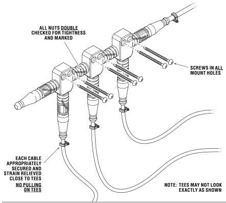
Figure 3-3. Correct CAN2 tee installation example.
