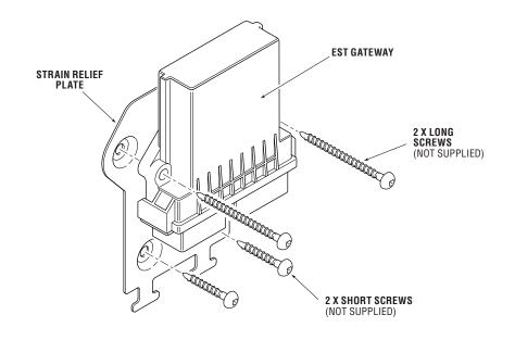
Figure 8-4. Gateway with strain relief plate.
