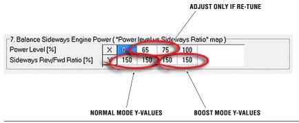
Figure B-13. Sideways REV/FWD ratio curve parameters.
