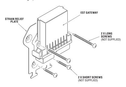
Figure 5-1 Gateway with strain relief plate.
