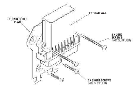
Figure 6-15. Harness connection to EST gateway.
