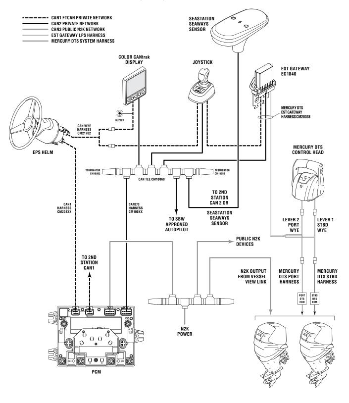
Figure 7-3. Mercury DTS – single station, twin engine.
