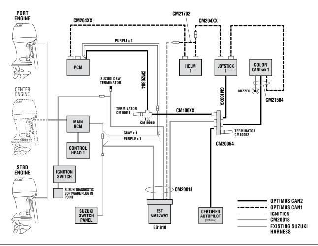
Figure 5-2. Suzuki EST single station, twin or triple engines.
