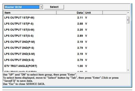
Figure 5-20. Service Data. Sample of typical values. SPC1 only.
