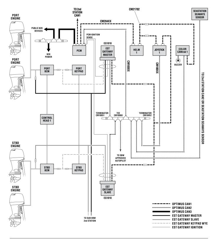
Figure 5-4. Suzuki SPC1 EST single station, quad engines.
