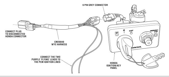
Figure 8-3. Honda IST – ignition line connection.
