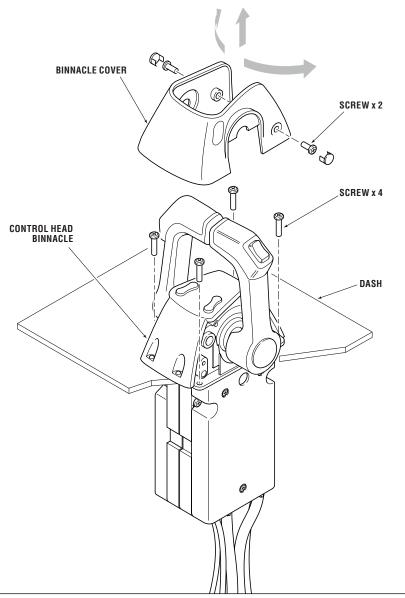
Figure 6-1. Control Head Binnacle removal.
