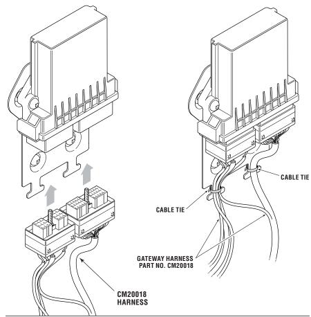
Figure 5-8. Harness connection to EST gateway.
