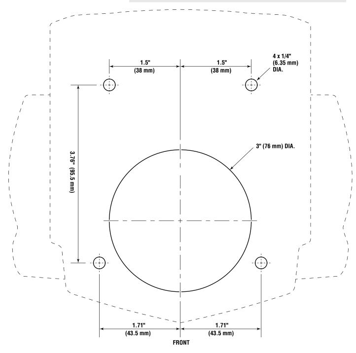
Figure A-2. Control Head Mounting Template.
