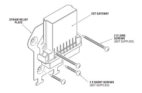
Figure 6-6 Gateway with strain relief plate.
