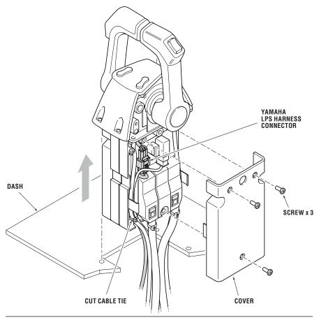
Figure 6-2. Cover removal and LPS harness identification.
