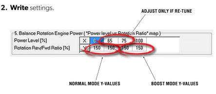
Figure B-11. Power level vs rotation ratio.
