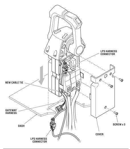
Figure 6-4. Cable tie and cover installation.
