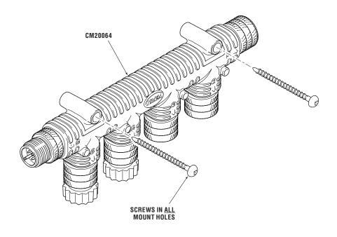
Figure 3-4. Alternative CAN2 6-port hub connection.
