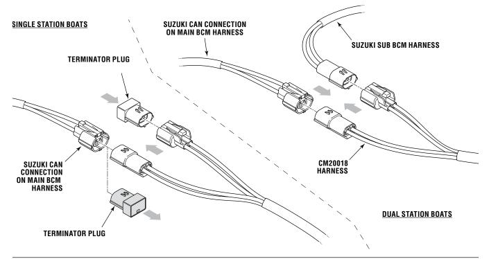
Figure 5-6. CM20018 connection to Suzuki CAN network.
