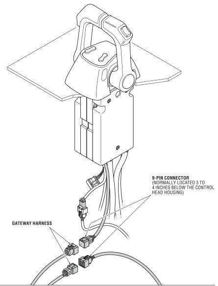
Figure 6-5. Status LED connector identification and connection.
