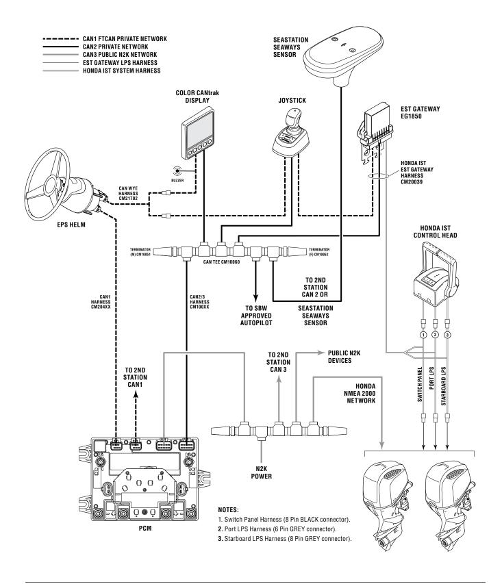
Figure 8-1. Honda IST – single station, twin engine.
