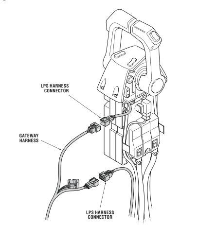
Figure 6-3. Gateway harness connection.
