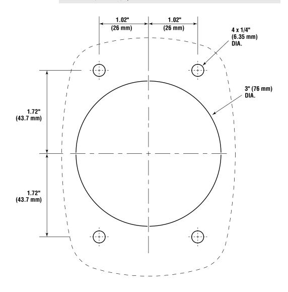
Figure A-1. Joystick Mounting Template.
