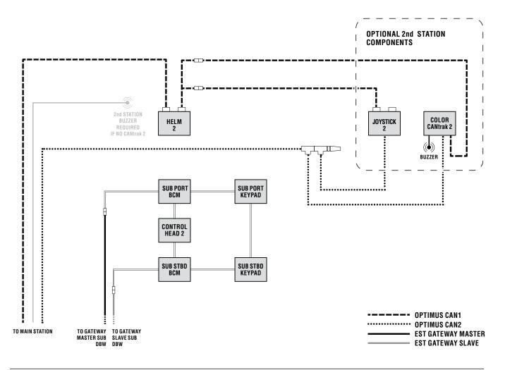
Figure 5-5. Suzuki SPC1 EST 2nd station, quad engines.
