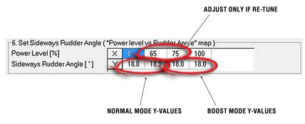
Figure B-12. Power level vs rudder angle.
