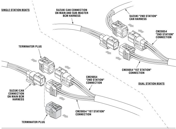
Figure 5-12. CM20054 connection to Suzuki CAN network.
