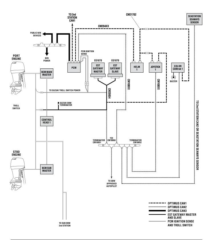
Figure 5-10. Suzuki SPC2 EST single station, dual, triple, quad engines.
