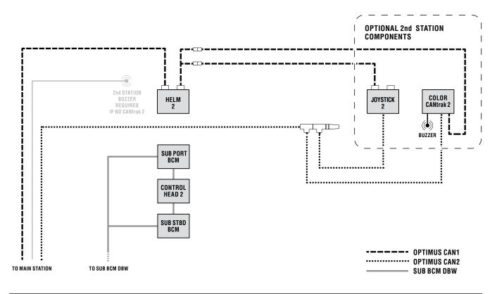
Figure 5-11. Suzuki SPC2 EST 2nd station, applicable for twin, triple, and quad engines.
