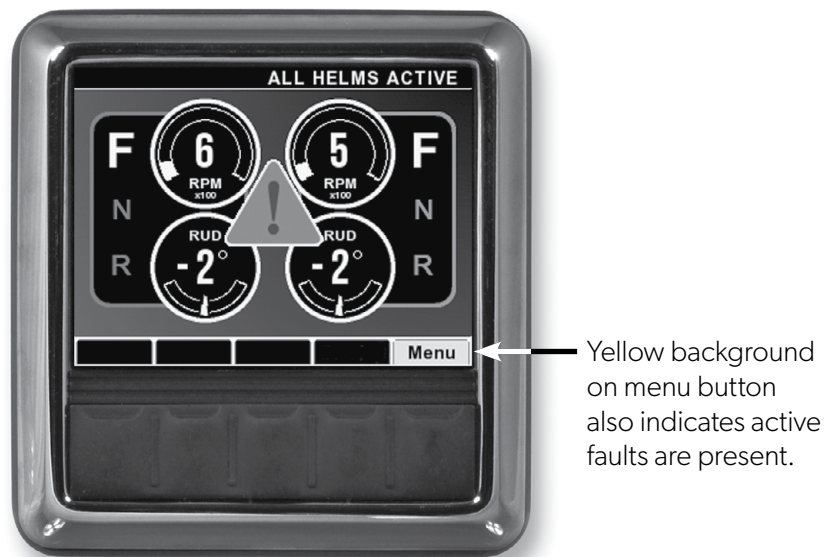
Figure 4-3. Run screen with system warning.
