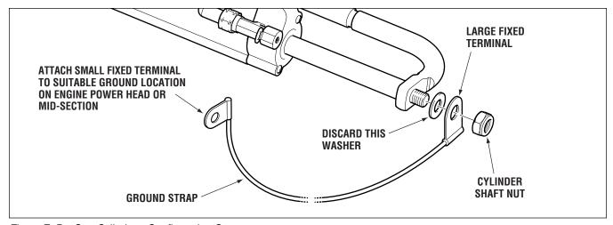
Figure E. BayStar Cylinders, Configuration C.
