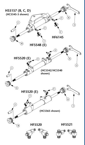
TYPICAL FRONT MOUNT TIE BAR KIT FOR HC5345-3 TYPE FRONT MOUNT CYLINDER HO6001/HO6002/HO6003
