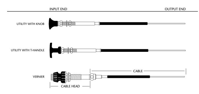
Note: The Marine Utility and Vernier control cable has a bare conduit at the output end with a .075 stainless steel wire.
