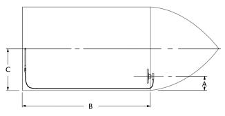
A single-cable, starboard drive push-pull mechanical cable system is shown in this diagram. If your mechanical system is different than the one depicted and/or you have any questions about mechanical steering after reviewing this guide, please contact SeaStar Solutions Technical Service.
