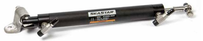
This cylinder is a light duty alternative to front & side mount cylinders. It is unbalanced with 5.5/6.5 turns lock-to-lock and fits engines with/without support (steering) tube. The splashwell mount cylinder is for single & multiple engine capability and has total power to 600 HP in counter rotating application. It can be transom or hull mounted cylinder. **NOTE: Not for use with SeaStar Pro helms.**
