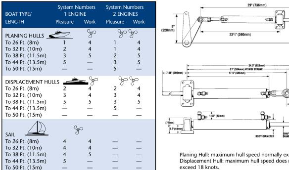
Planing Hull: maximum hull speed normally exceeds 18 knots. Displacement Hull: maximum hull speed does not normally exceed 18 knots.
