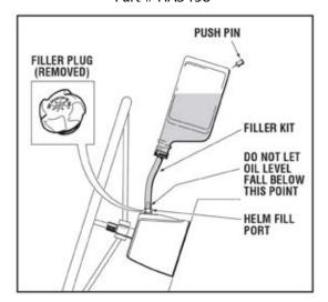
In an emergency, SeaStar EPS Fluid, any MD-3/4 rated ATF or MIL-PRF-5606H equivalent fluid that is filtered through a fine mesh screen can be used. The system MUST be thoroughly flushed as soon as possible with genuine SeaStar Steering Fluid after using an emergency fluid. In an EXTREME emergency, any non-toxic, non-flammable fluid that is filtered through a fine mesh screen may provide temporary steering.
