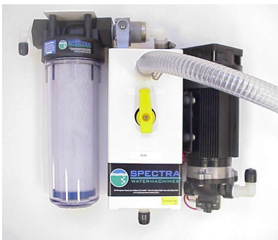
Service hose connected and service valve to SERVICE
